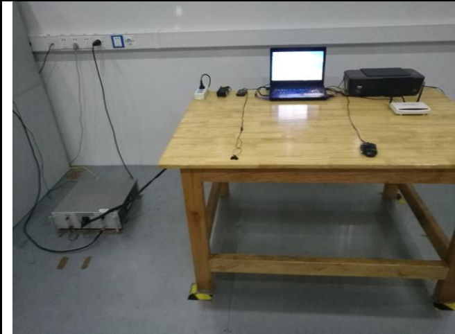
Conducted Emissions Test Setup – Front View
