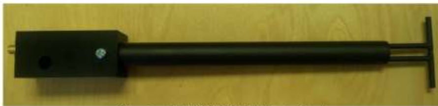
Figure 1 – MVG COMOSAR Validation Dipole
