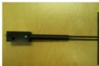
Figure 1 – MVG COMOSAR Validation Dipole
