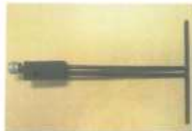
Figure 1 – MVG COMOSAR Validation Dipole
