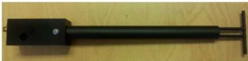
Figure 1 – MVG COMOSAR Validation Dipole
