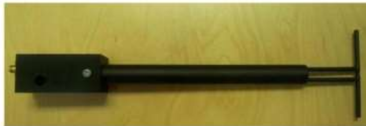
Figure 1 – MVG COMOSAR Validation Dipole
