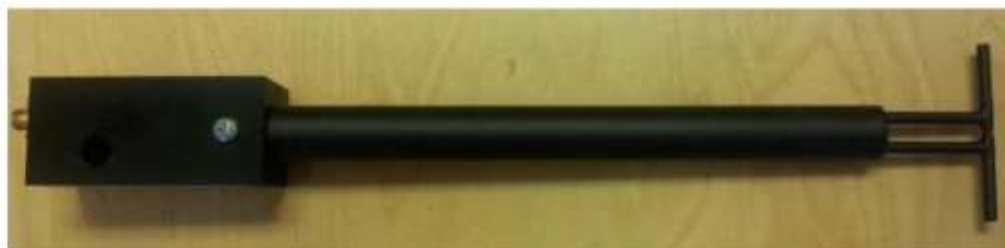
Figure 1 – MVG COMOSAR Validation Dipole
