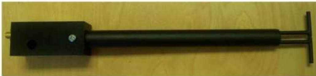
Figure 1 – MVG COMOSAR Validation Dipole
