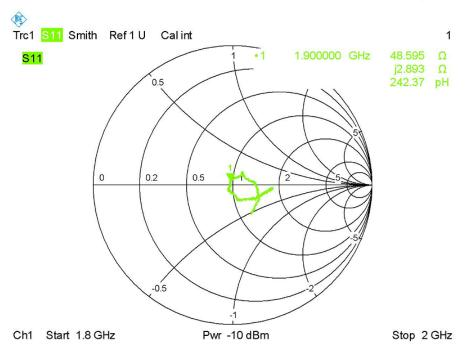
Calibrated return loss: -27.75dB; Measurement return loss: -28.54 dB(within 20%)
