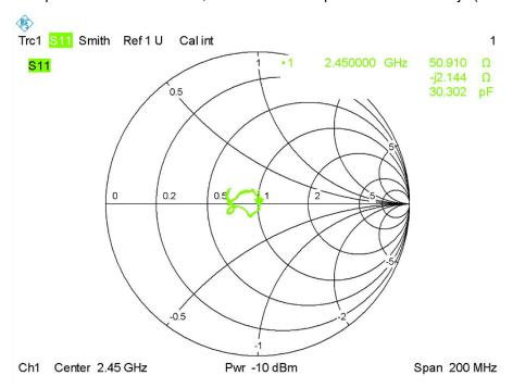
Calibrated return loss: -29.54dB; Measurement return loss: -31.08 dB(within 20%)
