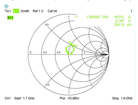
Calibrated return loss: -26.66dB; Measurement return loss: -27.3 dB(within 20%)
