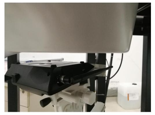
The antennal perpendicular with the back of device (separation distance is 25mm)
