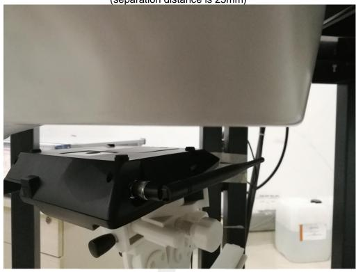
The antennal perpendicular with the back of device (separation distance is 25mm)
