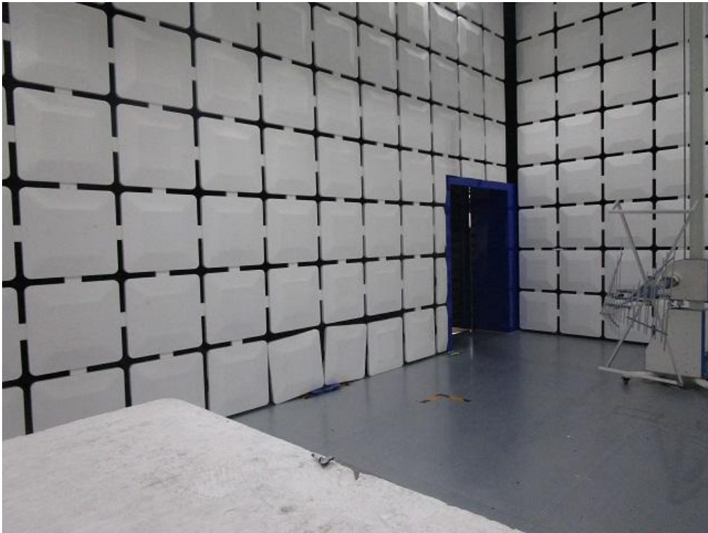
Description: Radiated Spurious Emission Test Setup
