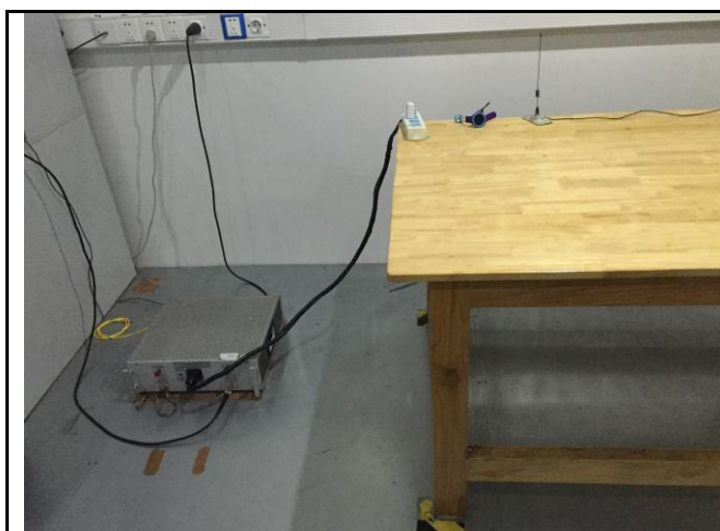
Conducted Emissions Test Setup Front View
