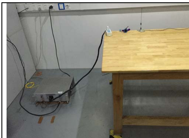
Conducted Emissions Test Setup Front View
