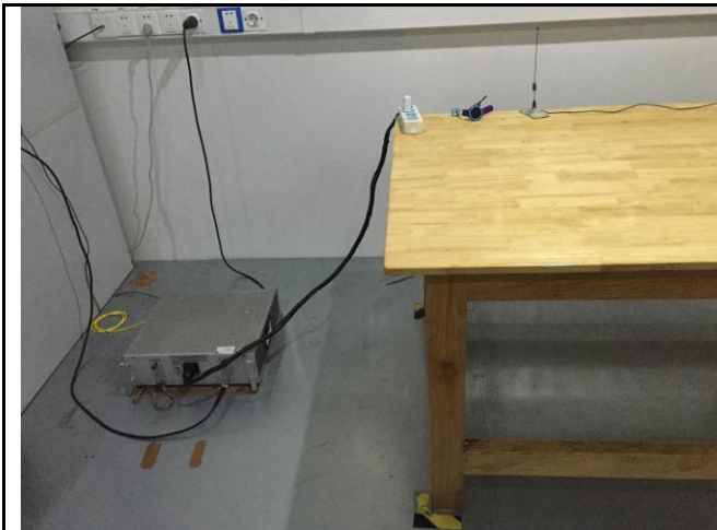
Conducted Emissions Test Setup Front View
