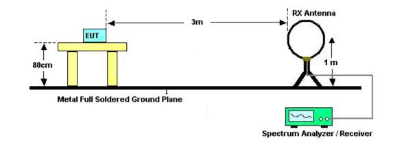
For radiated emissions from 30MHz to 1GHz
