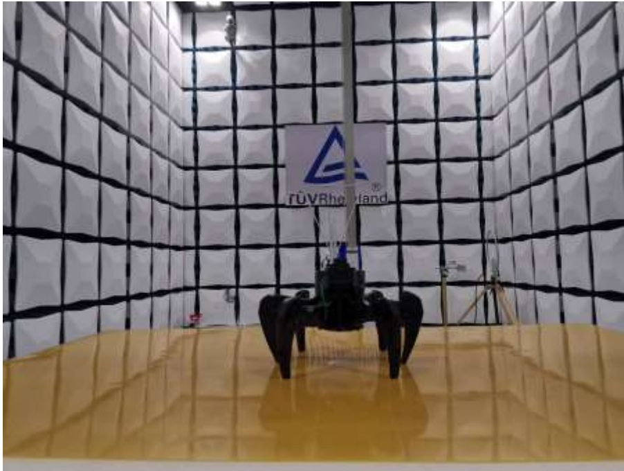
Photograph 1: Set-up for Radiated Spurious Emission, below 1GHz
