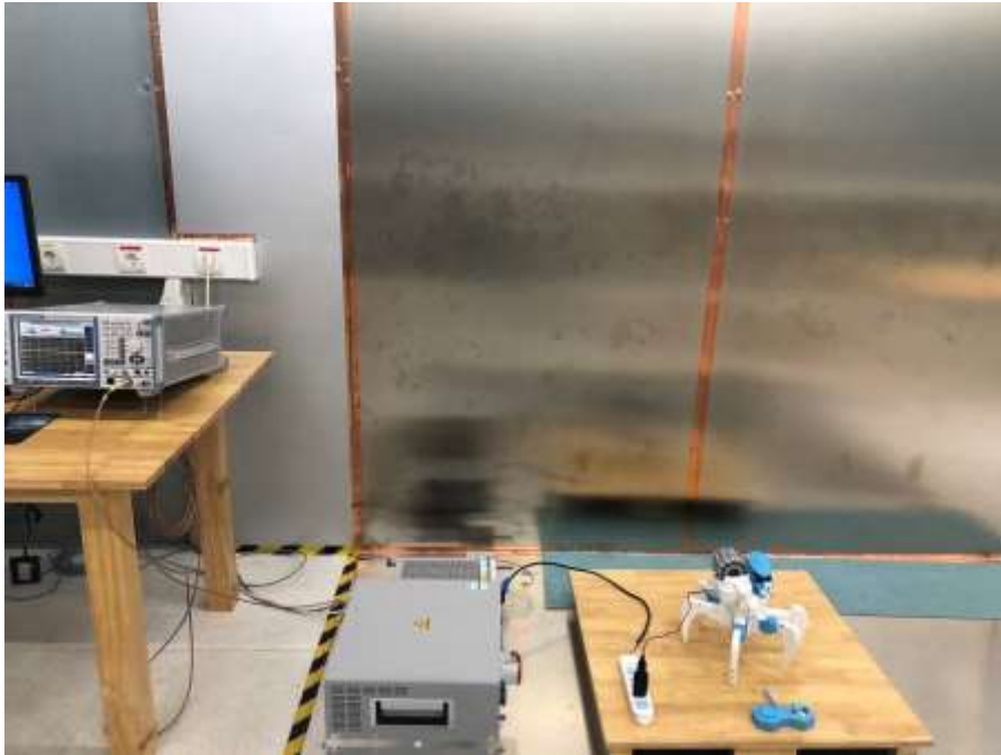
Photograph 3: Set-up for Conducted Emission on AC Mains
