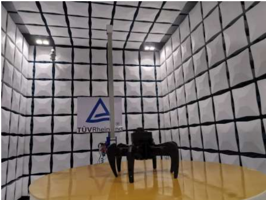
Photograph 2: Set-up for Radiated Spurious Emission, above 1GHz
