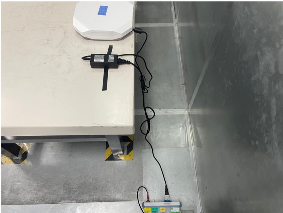
Description: Back View of Conducted Emission Test Setup for Power Port Test Mode 3
