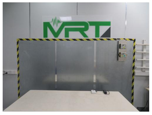
Test Mode 2 Description: Back View of Conducted Emission Test Setup for Power Port
