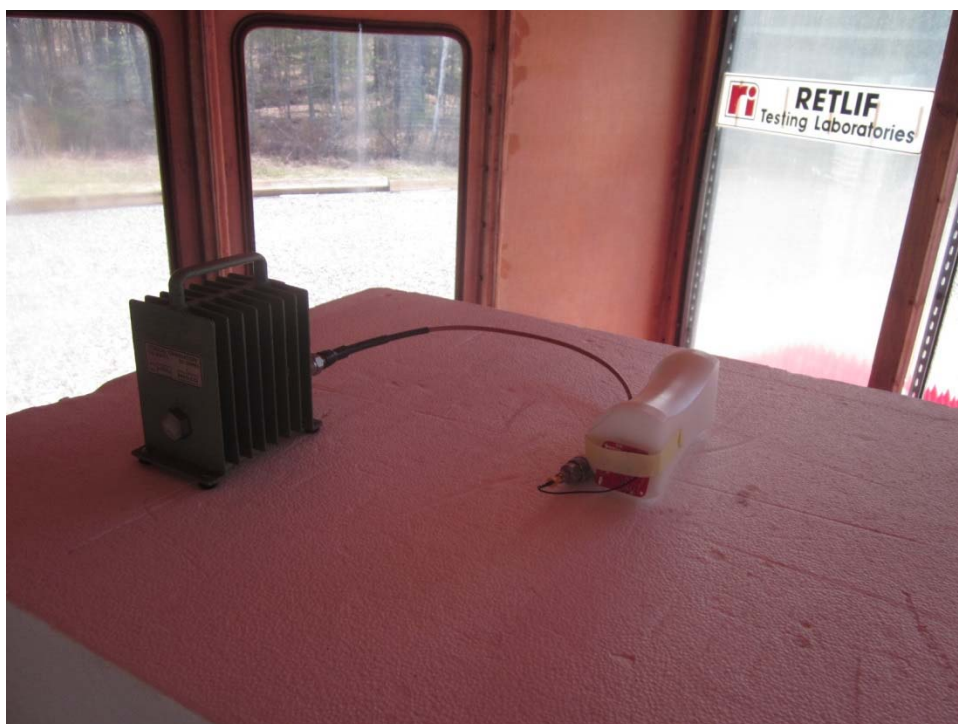
Test Configuration, antenna replaced with 50 Ohm Load
