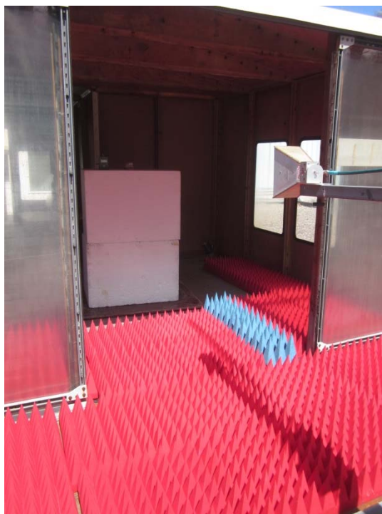
Horizontal Antenna Polarization, 1 GHz to 12 GHz, Double Ridge Guide Antenna
