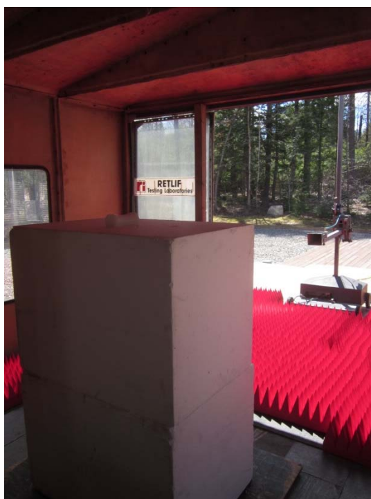
Vertical Antenna Polarization, 12 GHz to 18 GHz, High Gain Horn Antenna
