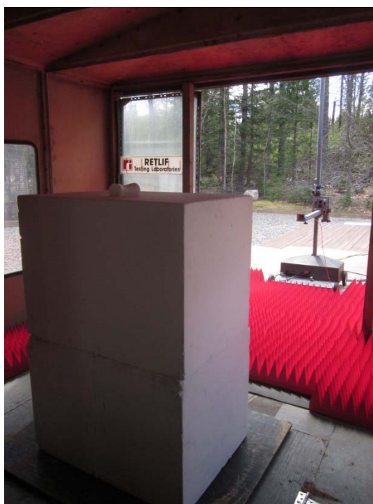
Vertical Antenna Polarization, 18 GHz to 25 GHz, Horn Antenna
