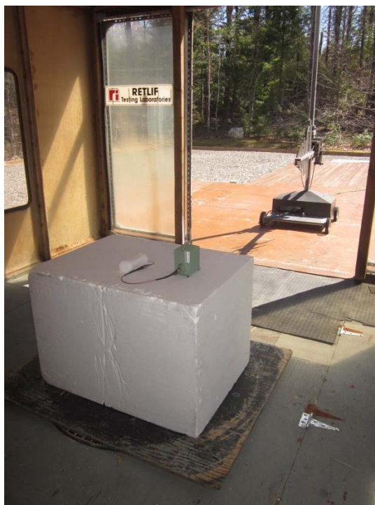
Vertical Antenna Polarization, 200 MHz to 1 GHz, Log Periodic Antenna
