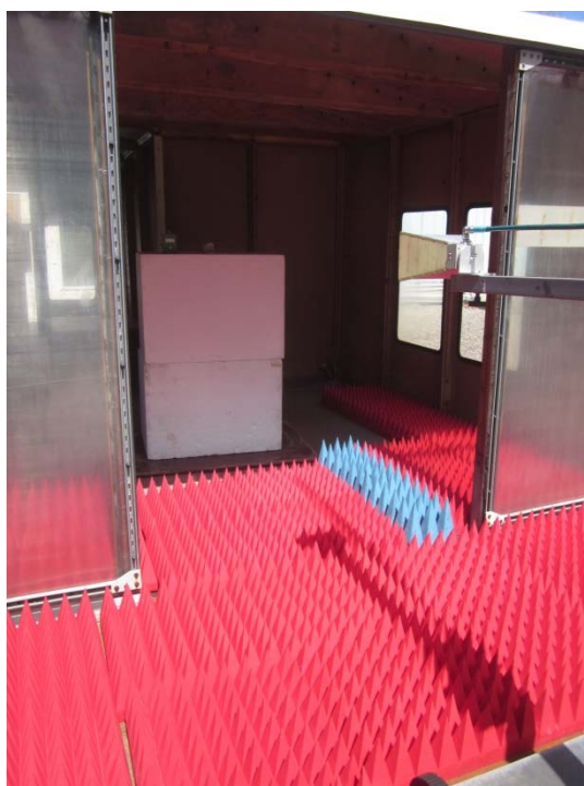
Vertical Antenna Polarization, 1 GHz to 12 GHz, Double Ridge Guide Antenna
