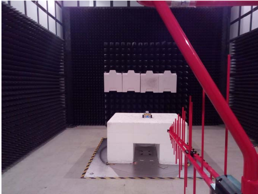
Radiated Emissions View (Below 1 GHz)
