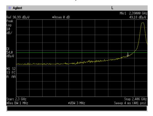
Restricted Band 2483.5 – 2500 MHz – Peak Tuned Freq = 2480 MHz
