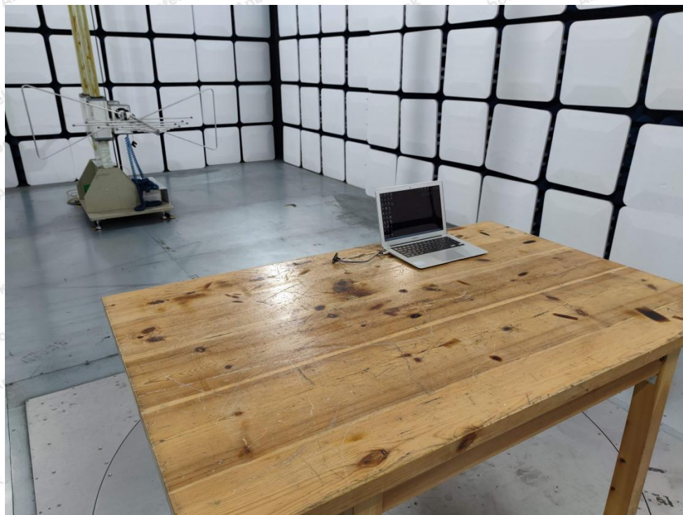
Photo of Radiation Emission Test
