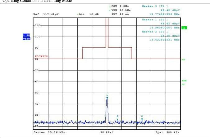
Note. To the above test data, the field strength level of 13.56 MHz is 44.62 dBuV/m and the worst limit subject to 15.225 (b) and (c) is 80.5 dBuV/m, so the EUT meets the requirement.
