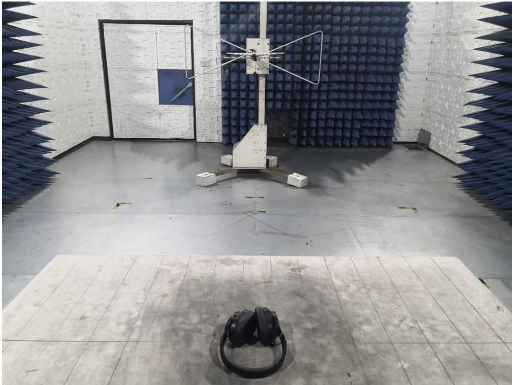
RADIATED EMISSION TEST SETUP ABOVE 1GHZ
