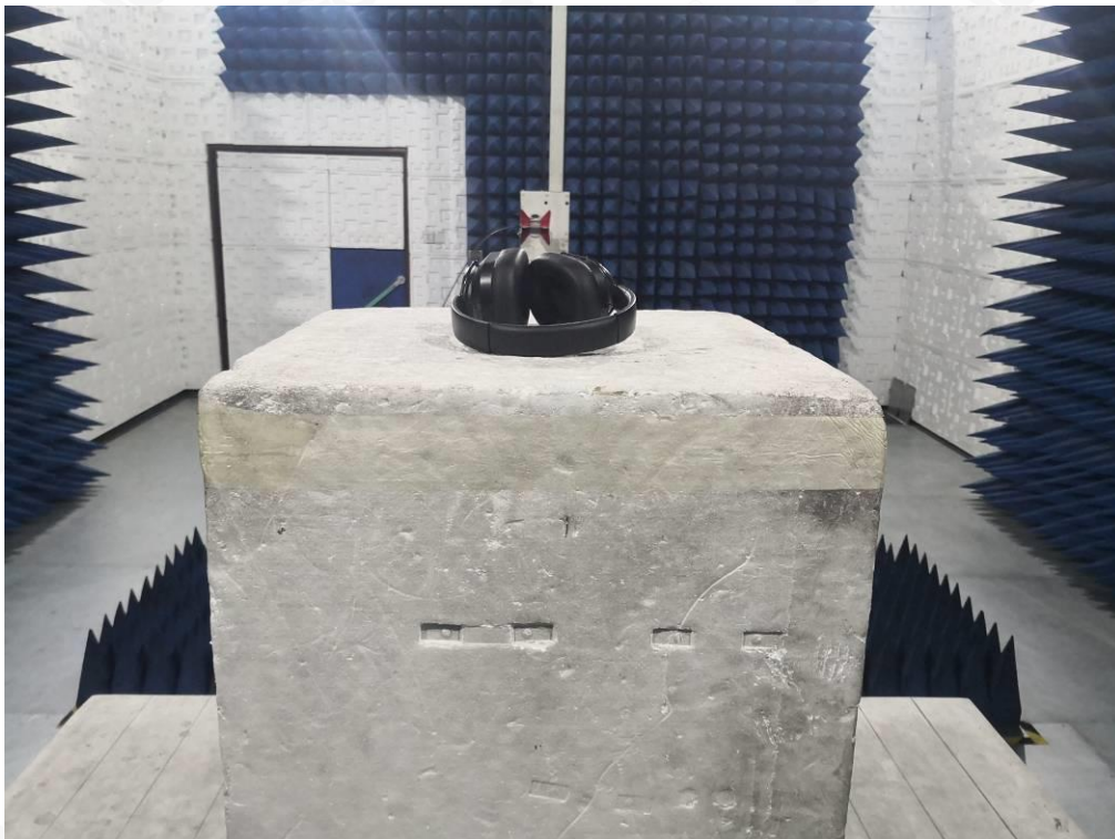
RADIATED EMISSION TEST SETUP ABOVE 1GHZ
