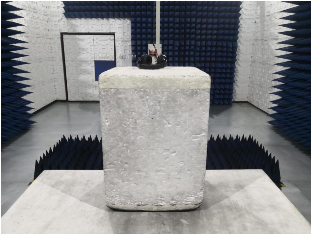
RADIATED EMISSION TEST SETUP ABOVE 1GHz
