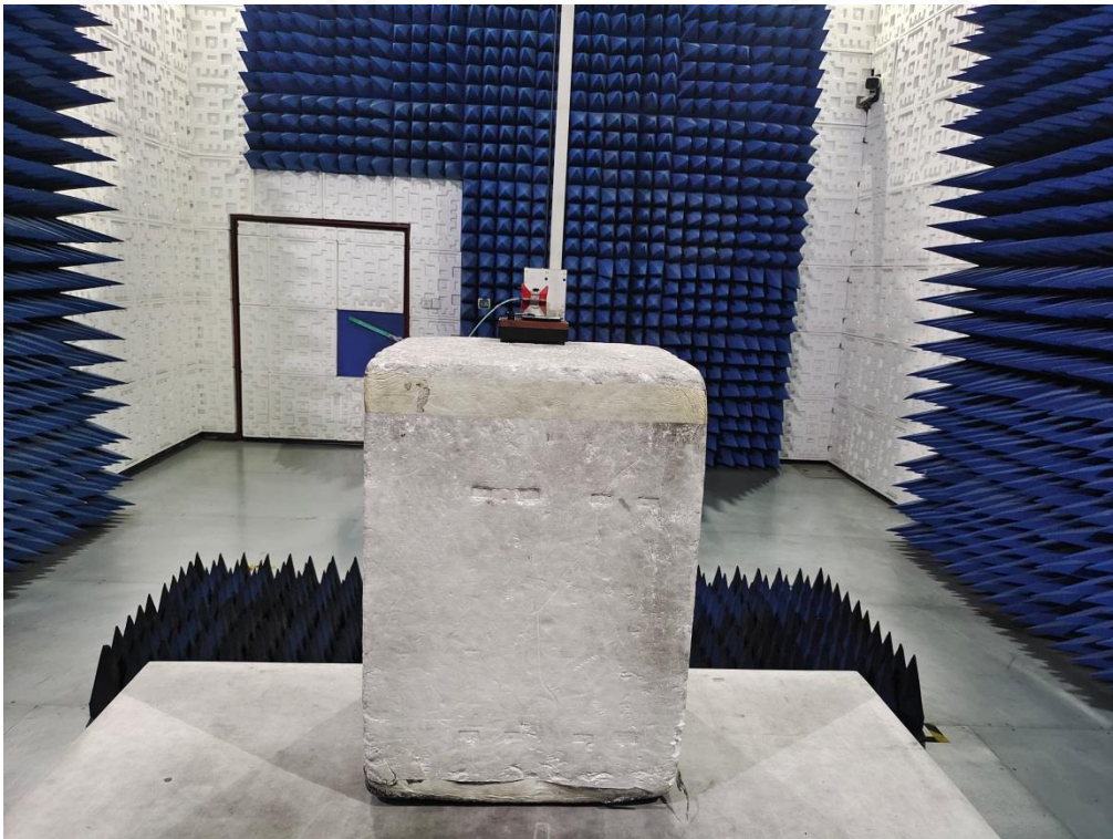
RADIATED EMISSION TEST SETUP ABOVE 1GHZ
