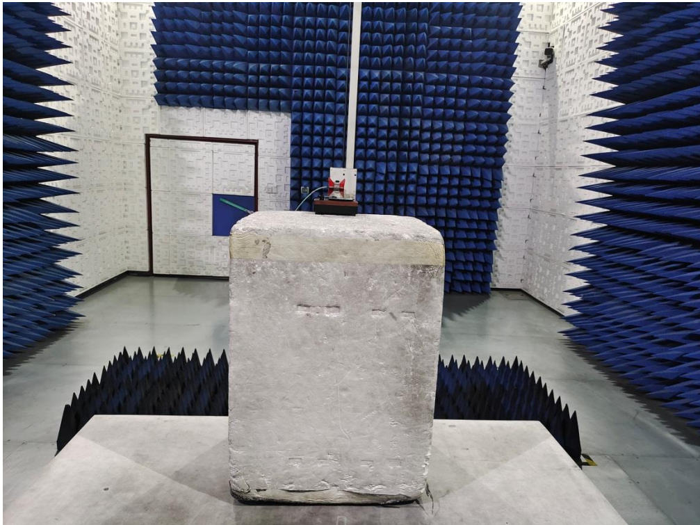
RADIATED EMISSION TEST SETUP ABOVE 1GHz
