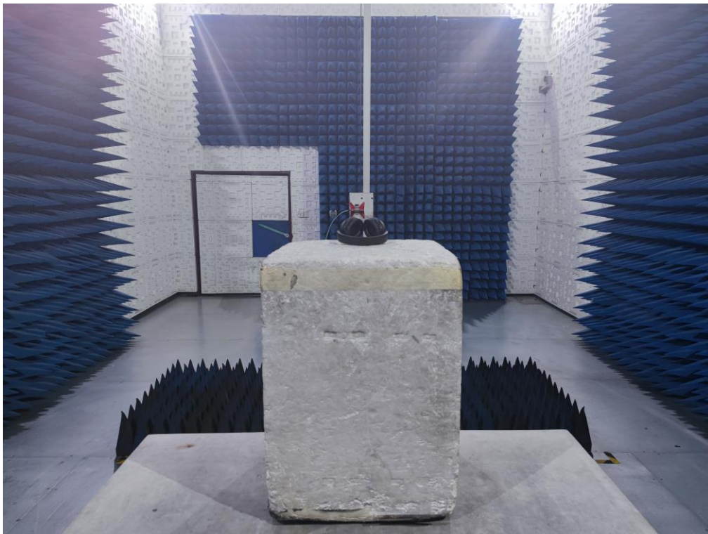
RADIATED EMISSION TEST SETUP ABOVE 1GHZ
