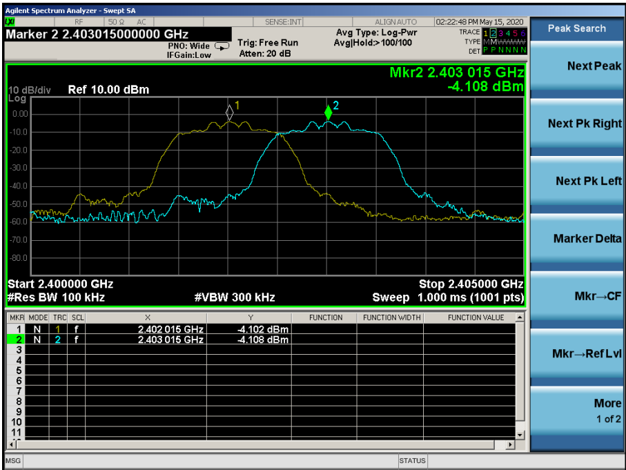
TEST PLOT FOR FREQUENCY SEPARATION
