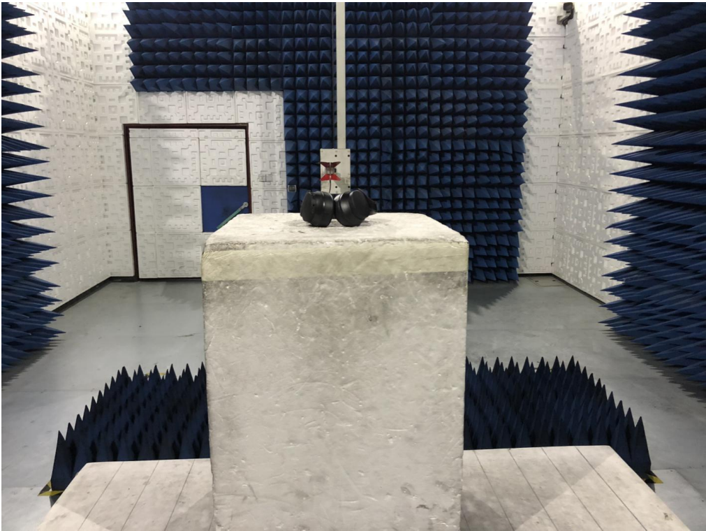
RADIATED EMISSION TEST SETUP ABOVE 1GHZ
