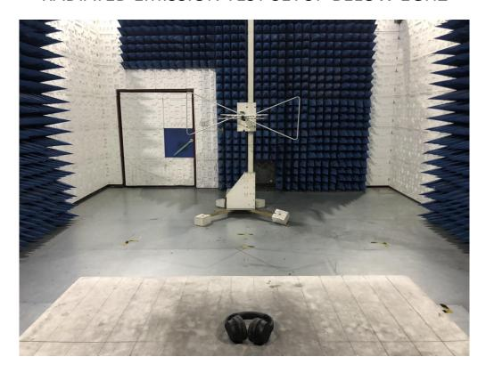
RADIATED EMISSION TEST SETUP ABOVE 1GHZ
