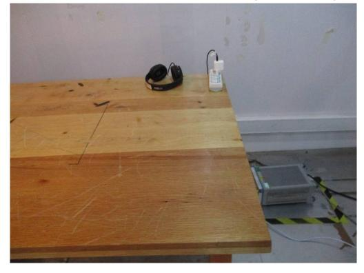
8.2 Radiated Spurious Emissions Test Setup
