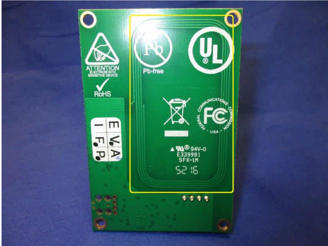
Photograph shows the EUT integral antenna (outlined in yellow)
