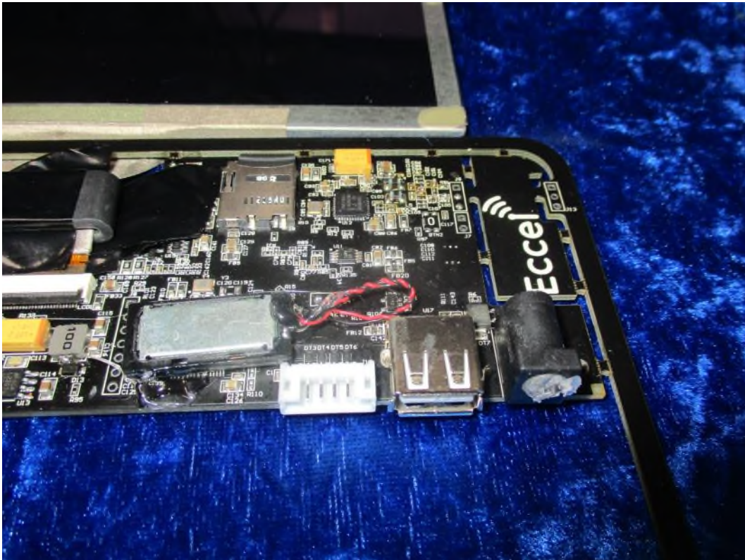
Photograph shows the debug port, and internal USB and DC sockets. The USB and DC ports are not accessible to the end-user. The applicant declares that the debug port is used for firmware / debug purposes only.
