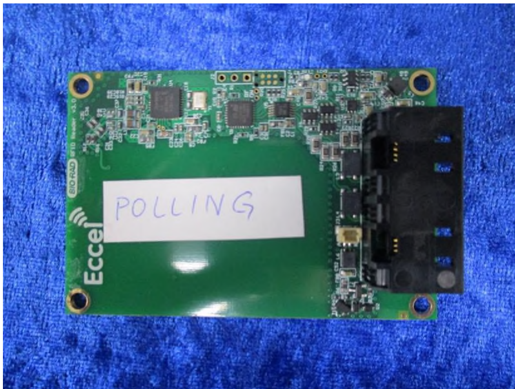
Board containing the 27h1 J8B crystal
