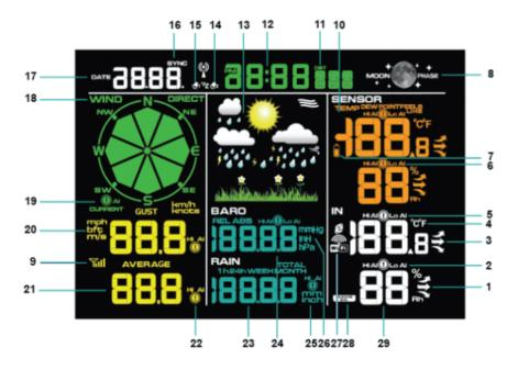
1.Indoor humidity change indication 2.Indoor humidity HI/LO alarm icon 3.Indoor temperature change indication 4.Temperature units (°F or °C) 5.Indoor temperature HI/LO alarm
