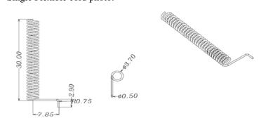
Inner copper size: 0.5mm Outer line size: 3.7mm
