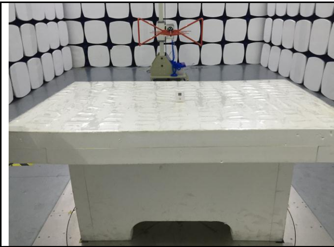
Radiated Spurious Emissions Test Setup Below 1GHz
