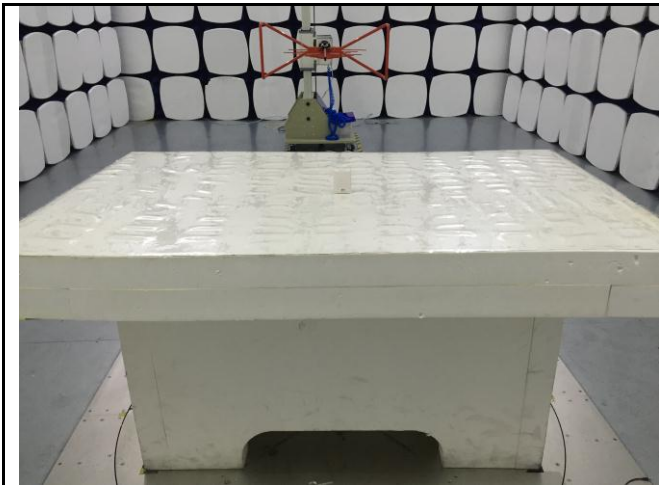
Radiated Spurious Emissions Test Setup Below 1GHz
