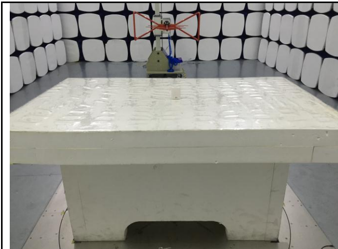
Radiated Spurious Emissions Test Setup Below 1GHz
