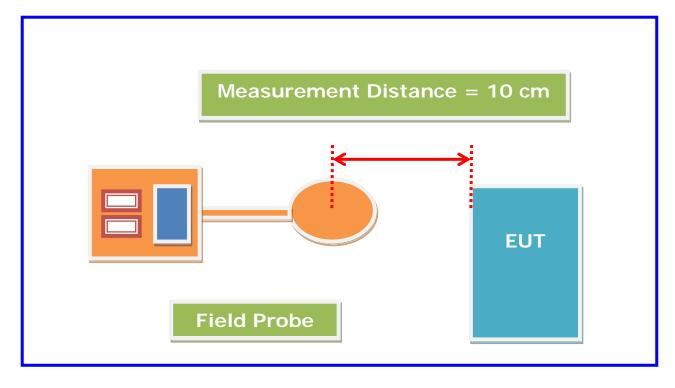
Measurements should be made from all sides and the top of the primary/client pair, with the 10 cm measured from the center of the probe(s) to the edge of the device.
