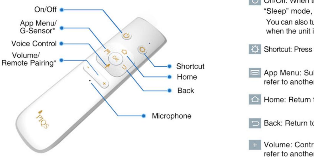
On/Off: When the unit is on, press once to select "Sleep" mode, "Reboot" or "Power Off".
