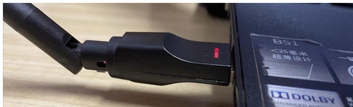
The reset is successful, remove the magnet and the red light is on
