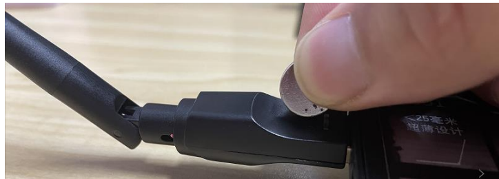
Place the magnet close to "Holyiot-21017" to reset it
