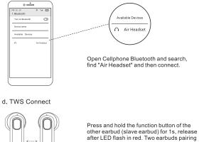
with each other automatically, the LED flashes in blue after connected (Default setting). (voice notice: TWS Connect)
