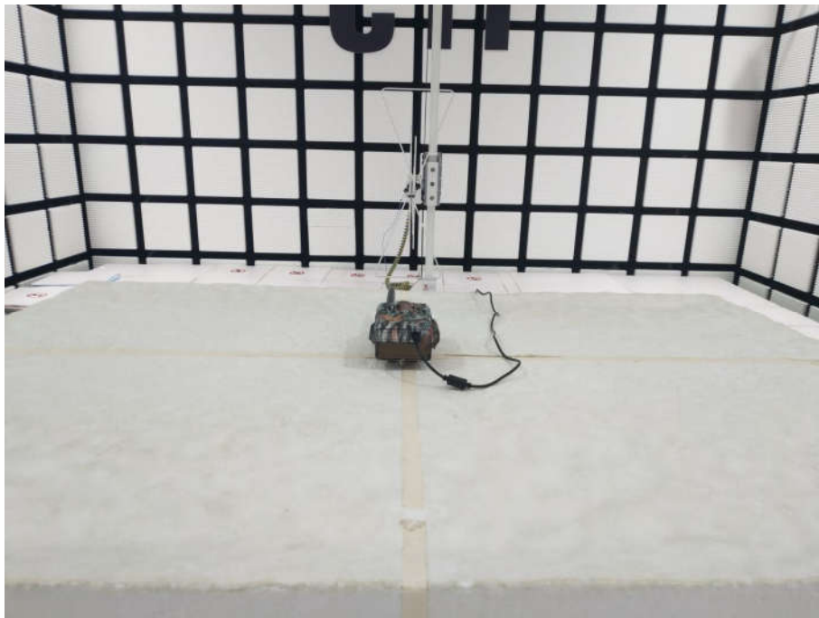
Radiated spurious emission Test Setup-1(Below 1GHz)
