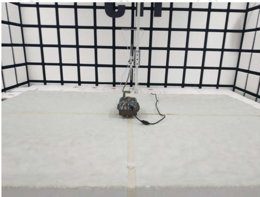
Radiated spurious emission Test Setup-1(Below 1GHz)
