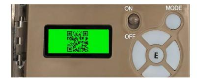
A QR code will appear on the camera display screen. Open your Strike Force Wireless app on your mobile device. Simply choose the "ADD CAMERA" option in the App located as a '+' symbol in the upper right corner of the 'Cameras' screen. A QR code scanner will appear on your screen. Scan the QR code displayed on the camera screen with your mobile device.
