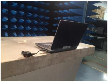
Configuration n°2: SteadXP+ connected to Laptop USB port , data enable.
