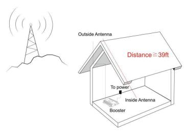
Plug the Power Supply into wall outlet then connect to Booster. The minimum distance between outdoor antenna and indoor antenna shall be more than 39ft, again.
