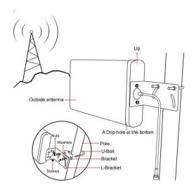
**Option C: Mount the Directional Outdoor Yagi Antenna**
