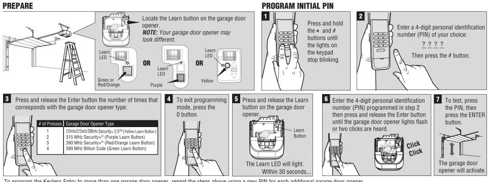
To program the Keyless Entry to more than one garage door opener, repeat the steps above using a new PIN for each additional garage door opener.
