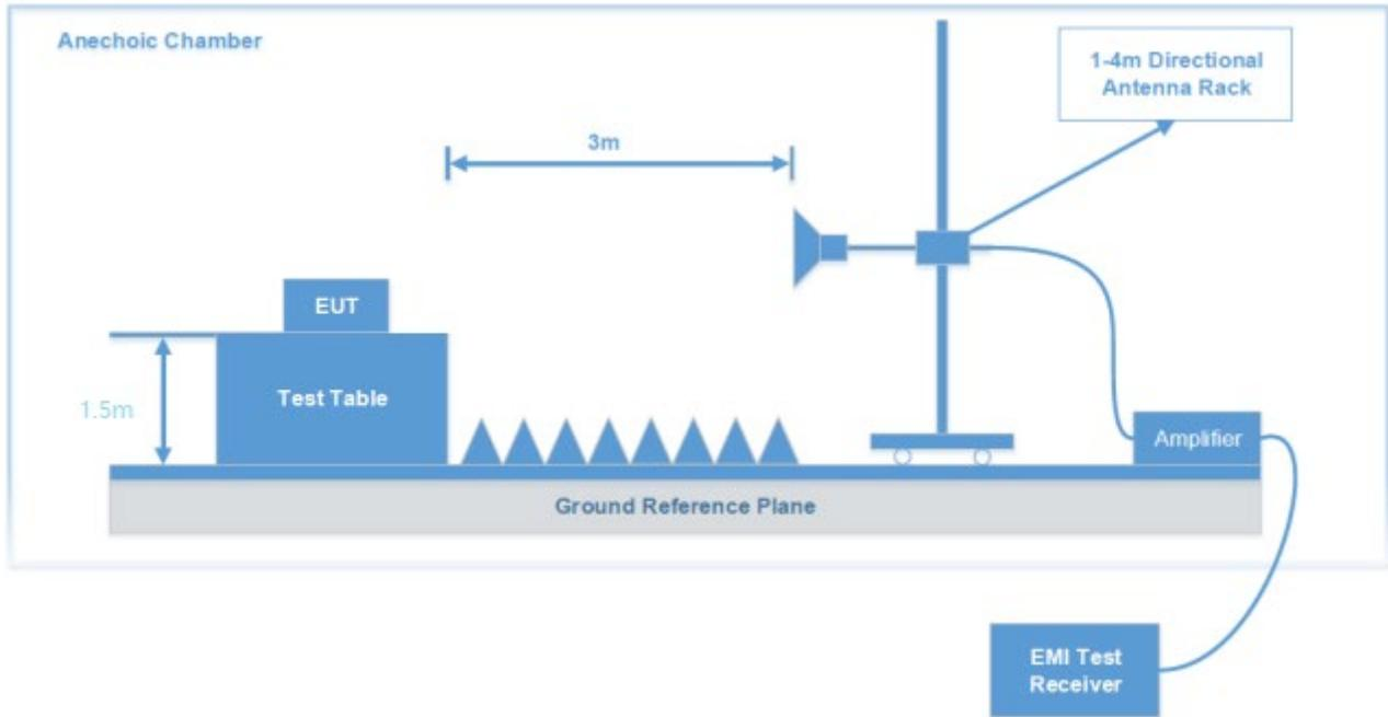
The radiated emission tests were performed in the 3 meters test site, using the setup accordance with the ANSI C63.10-2020. The specification used was the FCC § 15.205, 15.209 and 15.231.
