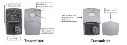
Step 3: Using a small screwdriver match the code to your receiver which was determined in step1. The switch has an on and off positions which is selected by pressing up or down. The 10 digit code on all remote controls must match what was selected in step 1.
