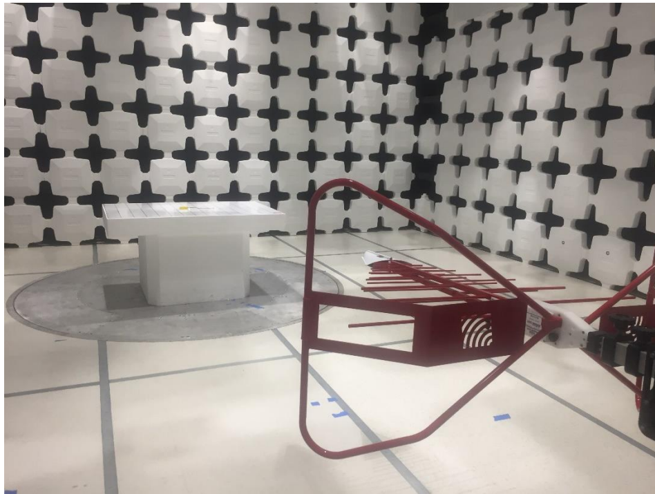
Radiated Emissions Below 1GHz setup – Front (flex model)
