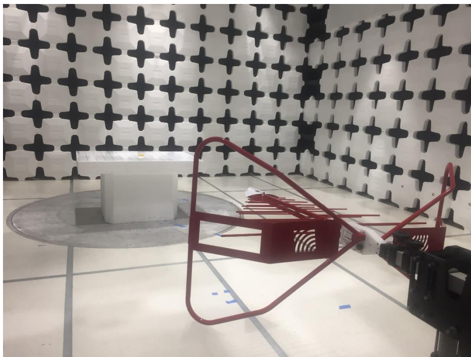
Radiated Emissions Below 1GHz setup – Front (non-flex model)
