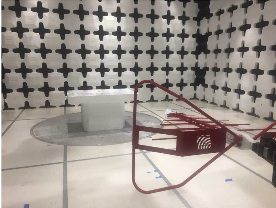
Radiated Emissions Below 1GHz setup - Front
